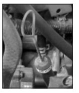
The automatic transmission dipstick has a red ring handle located in the rear of the engine compartment toward the center of the vehicle. See *Engine Compartment Overview on page 5-12* for more information on location.
